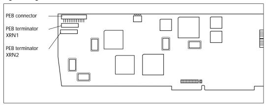
To remove a PEB terminator, place a flat-head screwdriver between the terminator and its socket and gently pry the terminator loose.
